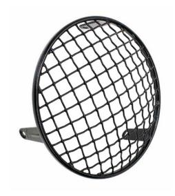
Robust injection molded headlight grill to customise the headlight and provide additional protection from debris. \*Not Homologated\*
